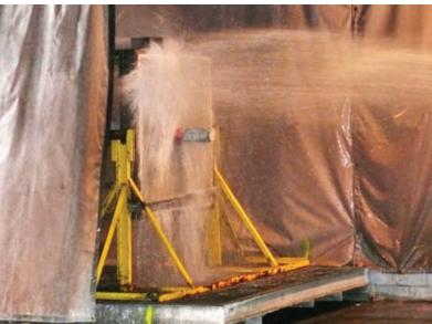
Figure 2 Assemblies are subject to a hose stream test to determine overall integrity.
