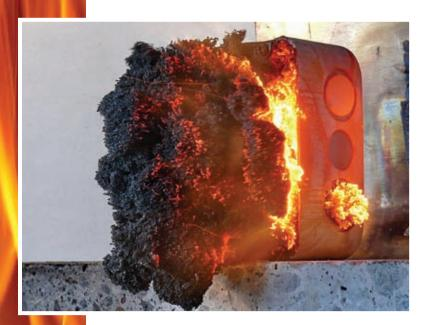
Figure 3 An intumescent electrical box insert
