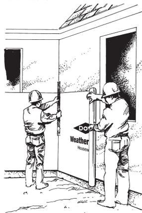
4. Overlap all vertical seams at least 6 inches. Overlap all horizontal seams at least 2 inches shingle fashion (the higher piece on the wall should lap over the lower piece). Taping is optional unless it is needed in an air barrier system design.
